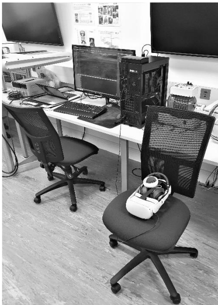
Figure 11. Listening test set up, with Oculus Quest 2 virtual reality headset and joystick.
