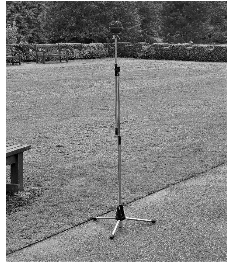
Figure 9. Zylia ZM-1 3 rd order ambisonic microphone position within the diffuse environment. This image does not show the microphone connected via USB.
