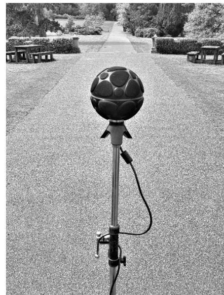
Figure 10. Zylia ZM-1 3 rd order ambisonic microphone Connected via USB within the diffuse environment, with orientation at 0 degrees forward.
